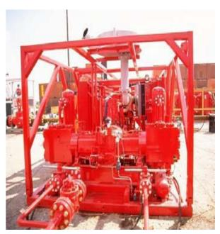
Figure 4: High pressure booster
