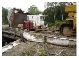
Figure 16: Tracked vehicle pulling equipment "sled" to site through the mud
