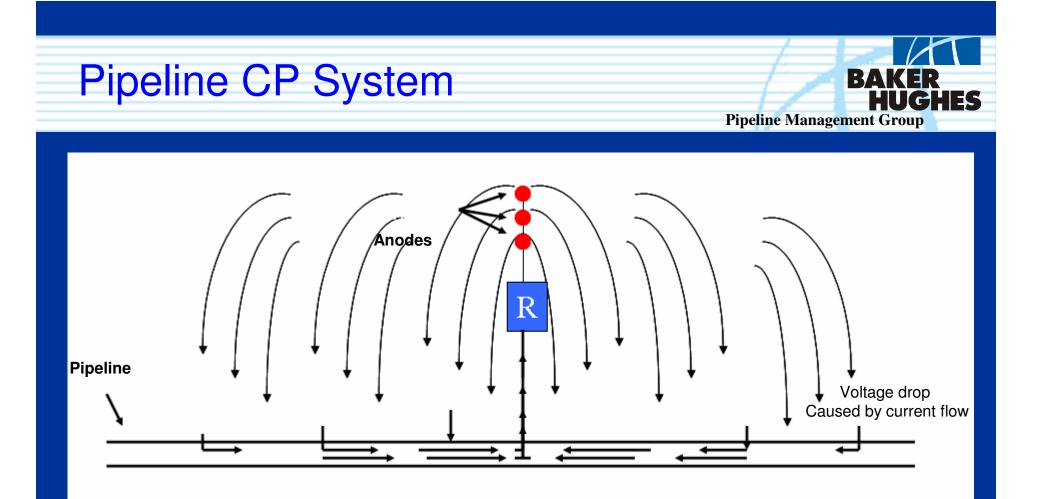
CP current is being "pushed" by the rectifier to the anodes where it enters the soil (electrolyte) then travels to the pipe surface where it enters the metal (cathode) and returns via a cable or other connection (negative).
