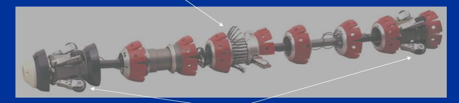
Tool reads and records voltage difference (both AC &DC) Between these two points.
