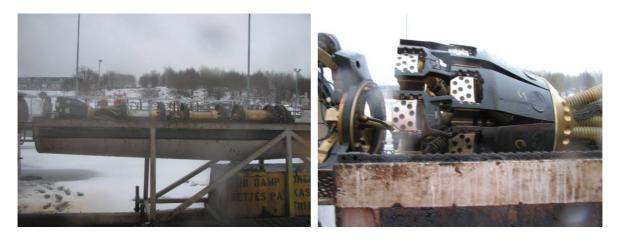
Receipt of clean 16" Ultrasound- based ILI after successful inspection of TOR1 pipeline at Mongstad
