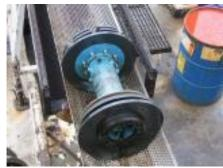
Disc Type pig with gauge plate
