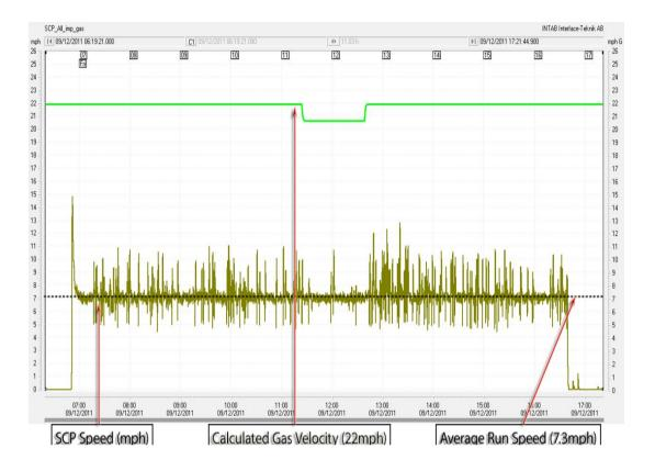
Figure 3.5: Gas Speed Velocity, SCP Speed
