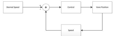
Figure 2.3: Closed loop control system
