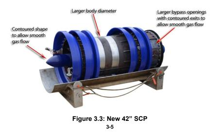
A control issue was also identified in these initial runs. This arose when the pig was slowing down either after the vanes had opened slightly or a change in terrain. In this circumstance the electronics did not react quickly enough and allowed the SCP to stop before the vanes started to close. To rectify this issue the control firmware was changed to speed up the reaction time.
