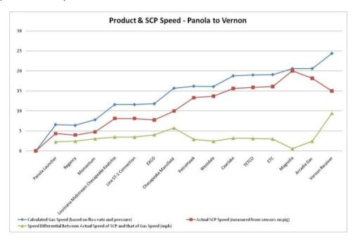
Figure 3.2: Gas and SCP speed
