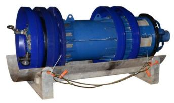
Figure 3.1: Initial 42" Speed Control Pig
