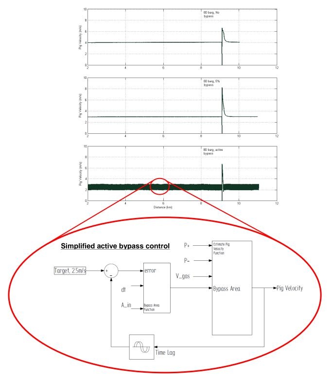
Figure 5, Comparison of no bypass, fixed bypass and bypass control
