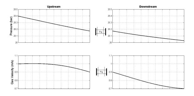
Figure 3, Pressure and gas velocity either side of the pig at a given time
