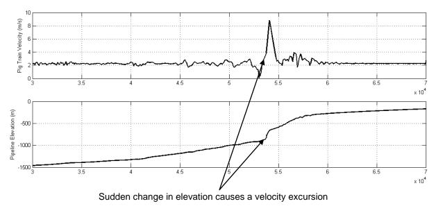
Figure 10, Output for 20" Gas Pipeline pig train velocity profile
