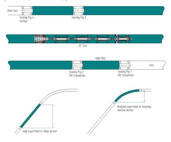
Figure 8, Example of an isolation pig train / effect of elevation
