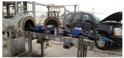
Figure 14: RRS - self-propelled metal loss inspection device
