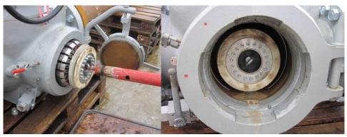
Figure 9: Pig Launch Valve
