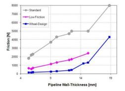
Figure 10: Dynamic friction force demonstrated for different cup designs
