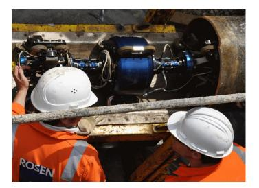
Field test with the RSS 16". Line was approximately 150 meters long and subjected to significant debris. Tool travelled in both directions.
