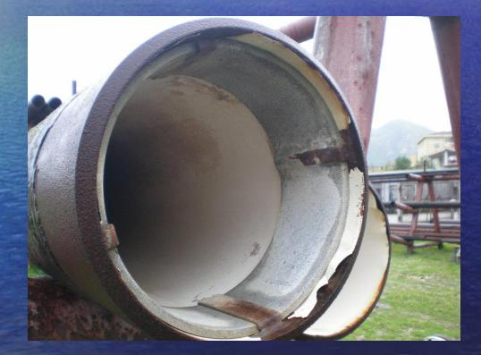
Internal Anodes On Similar Pipeline
