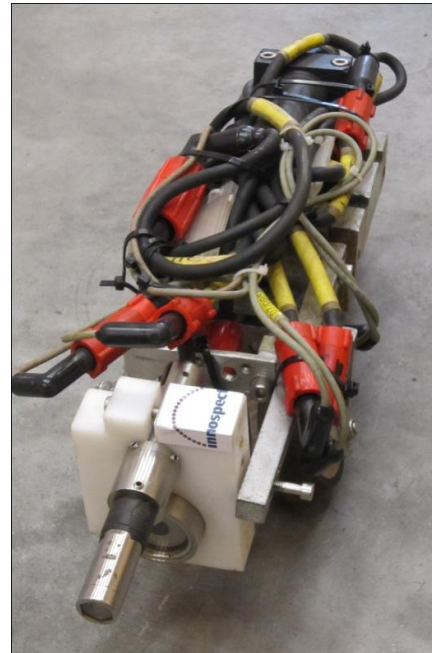
Figure 4: Left: The arm to mount the scanner on the hole. The scanner (right) could be lowered into the leg by the means of a steel rope. The pulley was inside the leg.
