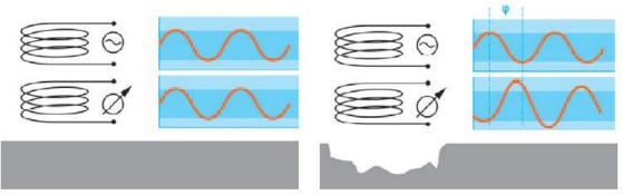
Figure 16: Principle of eddy current
