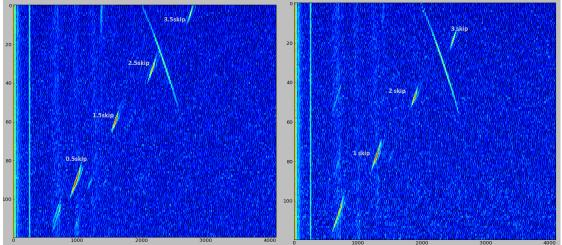
Figure 31: UT crack detection data for 16in pipe spool (left external, right internal)
