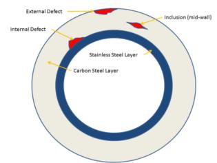
Figure 5: CRA Pipeline with defects
