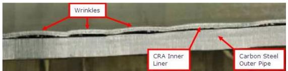
Figure 6: CRA Pipeline with defects (2)
