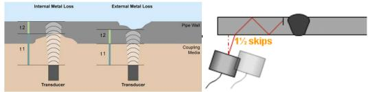
Figure 21: Ultrasonic principle (left metal loss, right crack detection)
