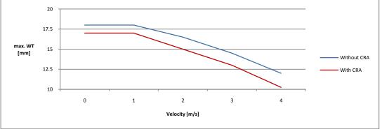
Figure 15: maximum wall thickness vs. tool velocity
