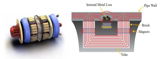
Figure 7: RoCorr MFL-A Tool and flux line distribution
