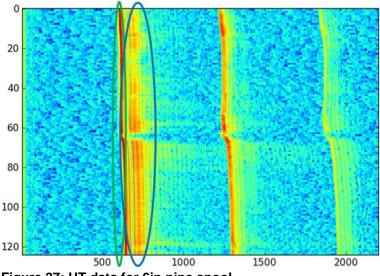
Figure 27: UT data for 6in pipe spool
