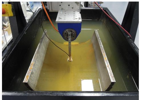
Figure 28: Test setup for test with ultrasonic sensors
