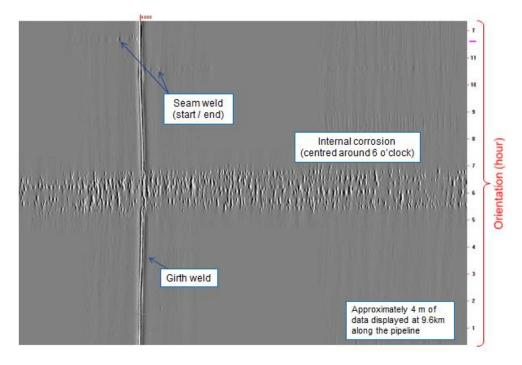
Figure 1 – Example of Metal Loss/Corrosion pattern present in the Pipeline
