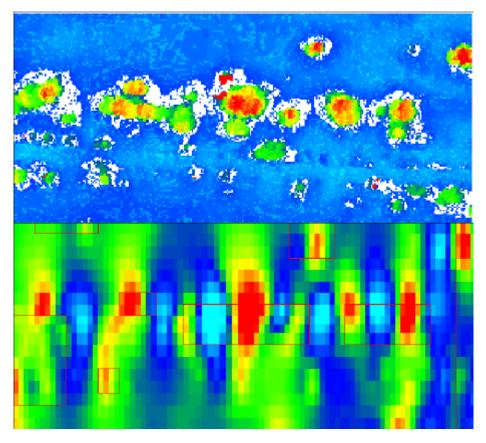
Figure 2 – Example DigCom Defect Matching: (AUT Data (Top) vs MFL (Bottom))
