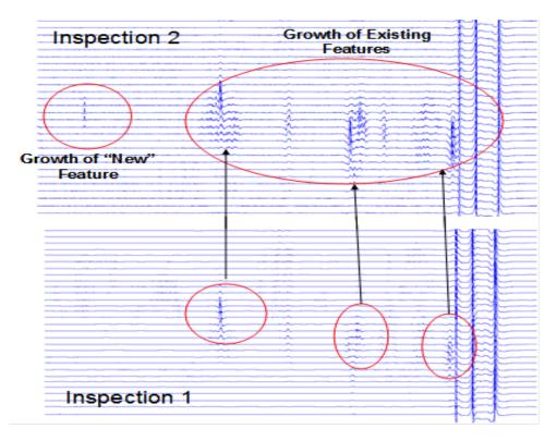
Figure 3: Detailed Corrosion Growth Assessment
