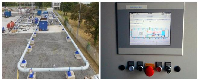
Figure 7: 12" test loop, total length of 150m with 453 (left); control panel for test loop (right)
