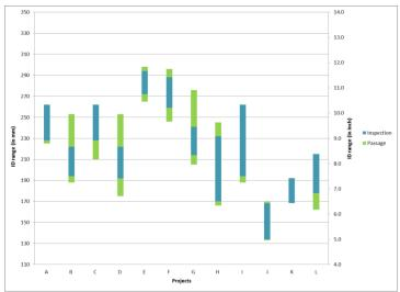
Figure 10: Pasage and inspection range for some offshore tools/projects recently developed by NDT Global.
