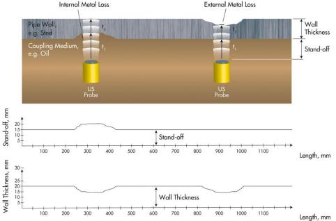
Figure 1: Schematic representation of UT wall thickness principle
