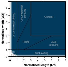
Figure 5: POF feature classification diagram. Colored area indicates application range of EVO Series 1.0 UM tools for detection, classification, and sizing with t = minimum {Wall thickness, 10mm}.
