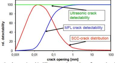
Figure 4: Ability of detection for cracks with different crack openings. Conventional UT crack tools show a significant higher detection ability for thin cracks than MFL technology.
