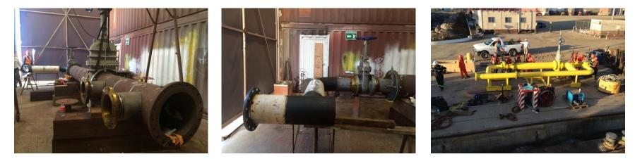
Design enables launching cleaning and MFL pig without intermediate spool recovery.
