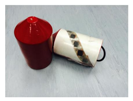
Image 2: 1<sup>st</sup> Generation foam pig. Sensors arranged in helical array. No PU cup was included in the design at this stage.
