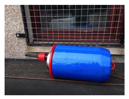
Figure 4: 2<sup>nd</sup> generation foam pig with PU disk bolted to the rear flange of the internal pressure vessel.
