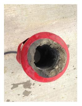
Image 3: Failures occurred when the internal pressure vessel blew through the nose of the foam. The foam body alone is not strong enough to hold the pressure vessel in place. This is especially the case for smaller diameter tools.
