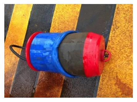
Figure 5: 2<sup>nd</sup> generation prototype. Damage to the outer PU coating due to the extra weight of the internal pressure vessel.
