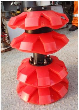
Figure 2: De-sanding pig
