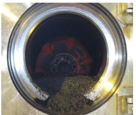
Figure 5: De-sanding pig and debris in receiver during pre-ILI cleaning Benefits of de-sanding pig use
