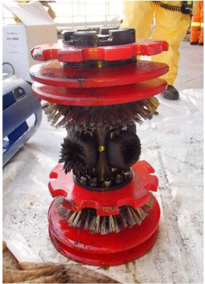
Figure 3: Brush pig with debris
