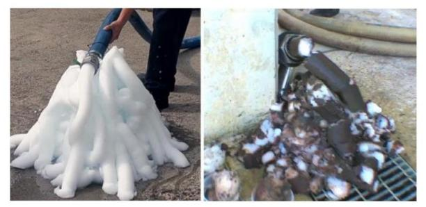
Figure 1 The ice slurry used in ice pigging is very thick and dry, whilst still flowable. It cleans tough deposits by abrasion.
