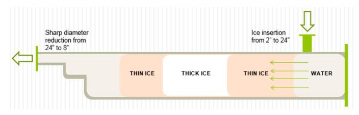
Figure 6, diagram showing how the ice slurry was injected to account for length to diameter ratio of the test rig.
