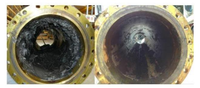
Figure 4 A 3m portion of the 24" pipe was loaded with 250 kgs of sand in one test, and 100 kgs of dyed petroleum wax in another, ice pigging cleaned both contaminants very effectively.
