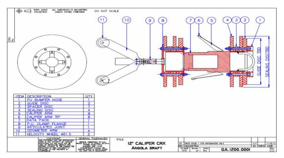
Figure 5—Segment W 12-in. caliper pig
