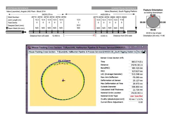
Figure 2—Data received from caliper survey of anomaly on Segment C
