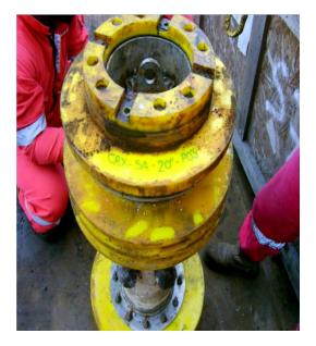
Figure 6—A 20-in. bi-di pig recovered from Segment A
