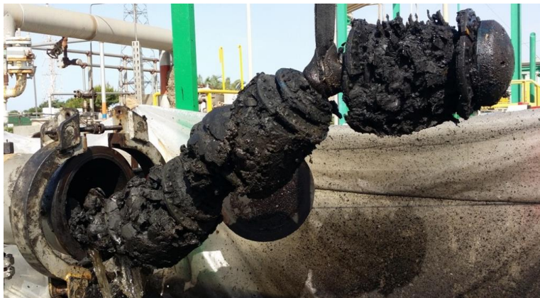
Pathfinder Run Shows Distribution of Wax Thickness Along the Line
