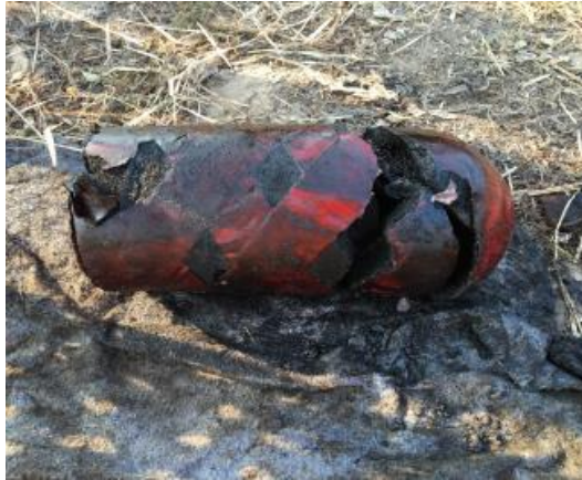
Foam Cleaning Pig Damage
