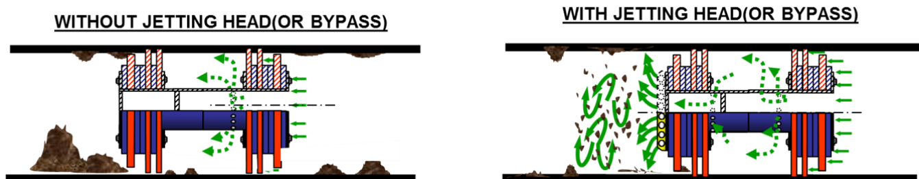
Figure 3: Effect of bypass on debris
