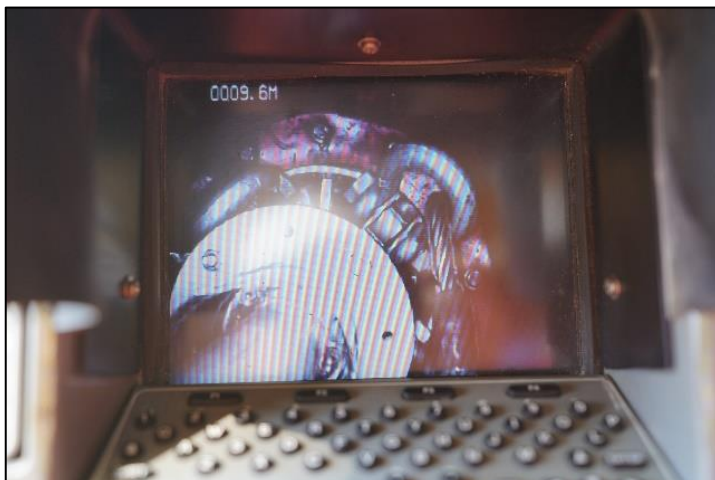
Figure 13: Camera monitor showing tool connected to the pig
