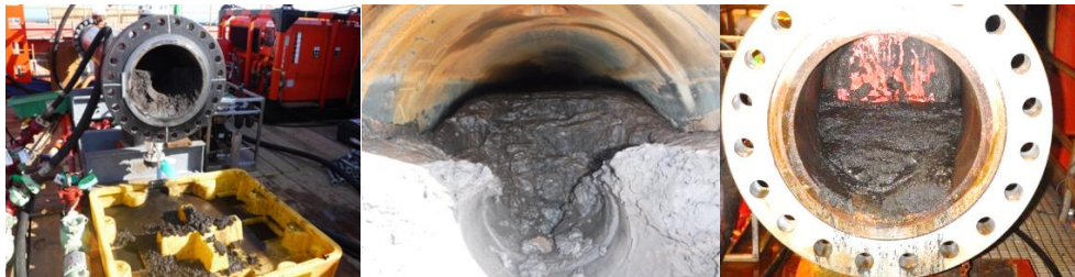
Figure 3: Examples of debris displaced by cleaning trains
