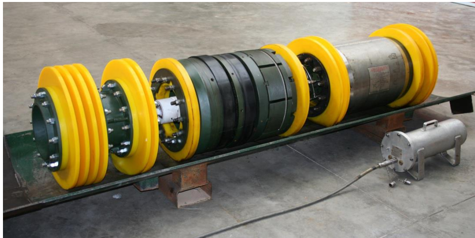
Remote Control Tecno Plug® In Pigging Configuration
