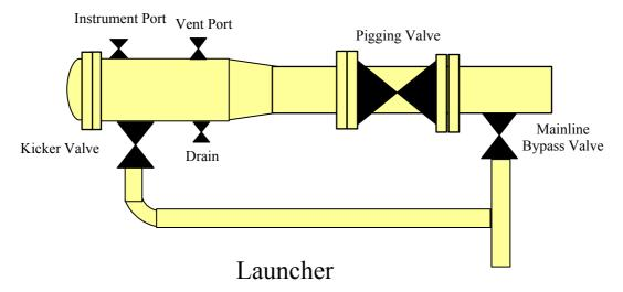
Again the same pig train can be launched from a multiple-pig pig trap by redirecting flow through pipework to allow individual pig launching as in the sketch below.
