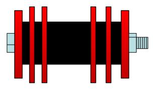
Similar to the mandrel pig, the elements are fitted to a single bolt, rather than a solid body.
