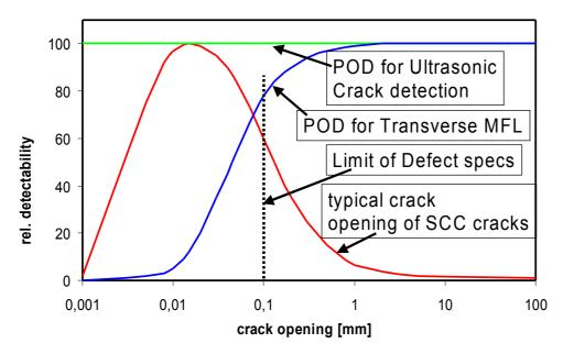
Figure 3: The use of MFL crack detection is limited in case of SCC, where the crack opening is usually to small.
