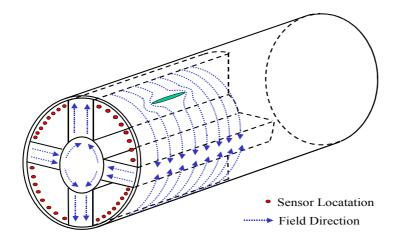
Figure 2: The transverse MFL Principle
