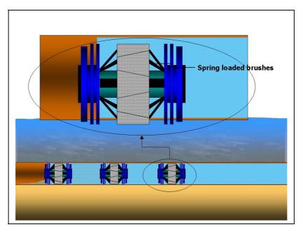
Fig. 1 – Cleaning and Filling a New Pipeline
