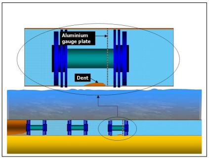
Fig. 2 – Gauging a New Pipeline
