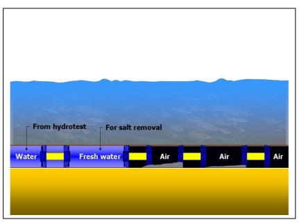
Fig. 5 – Dewatering a Gas Pipeline
