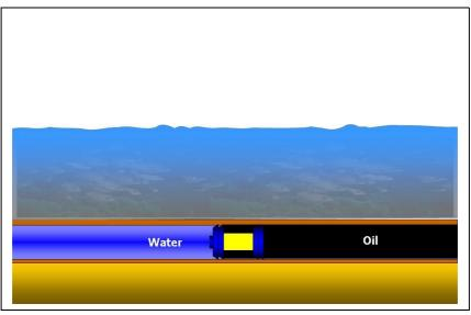
Fig. 4 – Dewatering an Oil Pipeline
