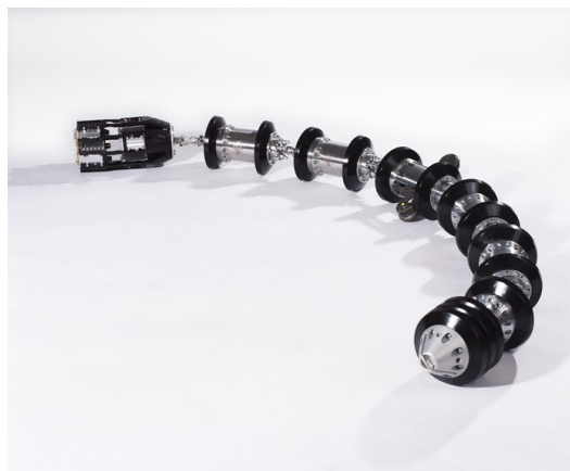
Figure 6: 6" configuration of the ultrasonic wall thickness measurement tool (LineExplorer).
