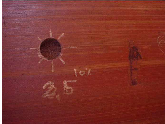
Figure 4a: Photograph of a circular defect of 25 mm
