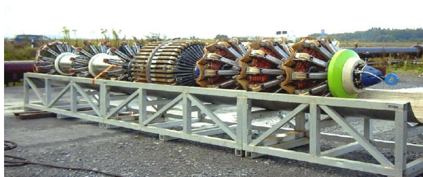
Figure 2: MagnoSurveyor metal loss survey tool ready for launching.
