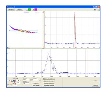
TFI tools are very useful for locating & sizing zones of small longitudinal cracks. A zone of very severe longitudinal cracks, being 60% p.w.t., was precisely located and assessed, using TFI technology. This zone was detected in a Russian trunk gas pipeline.
