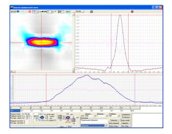
Now the problem of discrimination in identification of mid-wall laminations and SCC cracks is solved. Statistically, nearly 95% of such mid-wall laminations are opened in the inner pipe wall, only insignificant number of such cracks being opened in the outer pipe wall. The longitudinal crack is clearly seen on the colored TFI inspection plot.
