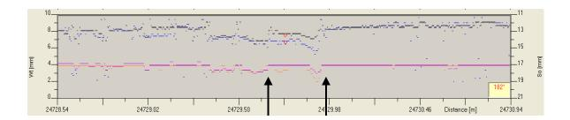
Figure 5: Sample data of a depth profile obtained in a section of channeling corrosion. The upper two lines show the wall thickness of two measurements that are two years apart. The lower line show the stand-off readings. The growth is found only at a specific spot.
