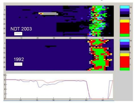
Figure 4: Pixel-by-pixel comparison of a metal loss defect. No change is found.
