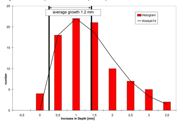
Figure 2: The increase in depth for 89 sample pairs of metal loss features as a histogram. There is a deviation of the mean from zero, that cannot be explained by the pig measurement uncertainty alone.
