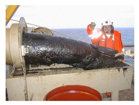
Figure 1 Part of a wax plug retrieved from the pig trap at Statfjord B after pigging the pipeline from Snorre B to Statfjord B (Sept. 2001)
