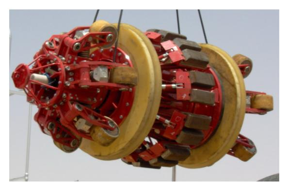
Figure 2: ROSEN 48" Black Powder Cleaning Tool before launching
