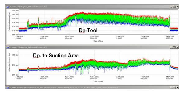
Figure 5: Differential pressure at cleaning tool and suction system
