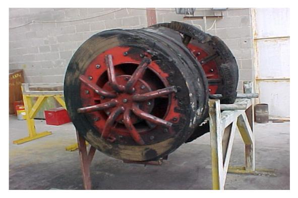
Figure 1: Cleaning tool after a 50-km inspection through black powder.
