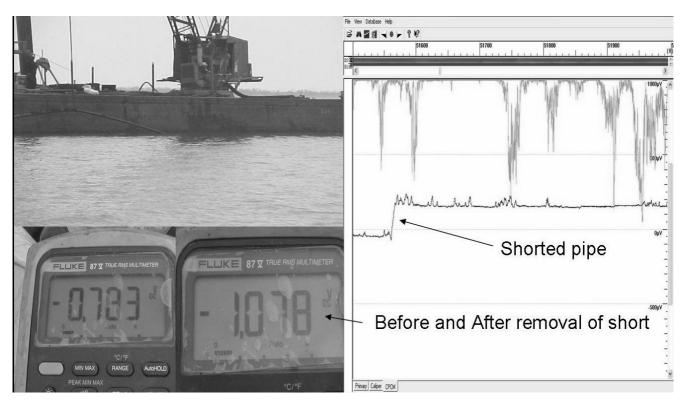
Figure 5- Pipe to soil potential before and after shorted pipe was removed
