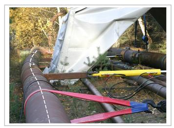
Figure 1: 4-point bending with hydraulic jacks
