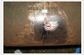
*Figure 4: Integrated strain gauge (red circle) for external strain measurements*
