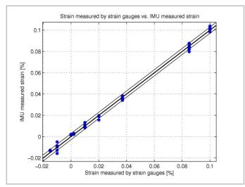
Figure 7: Strain gauge readings plotted against IMU strain results
