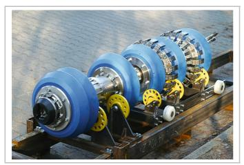
Figure 3: 16" RoGeo·Xt with XYZ mapping and HiRes ID mapping module
