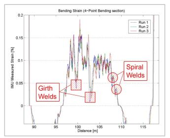
Figure 6: Data distribution typical of a strain area (several strain layers)
