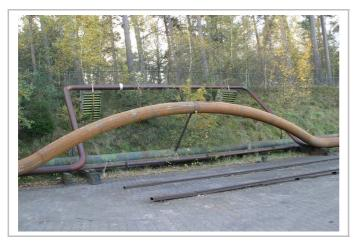
Figure 2: 5D-25D-5D bend section simulating plastic deformation
